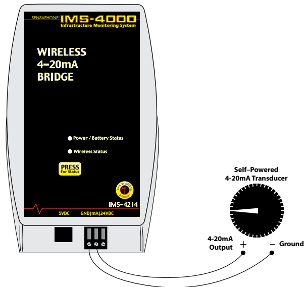
4-20mA sensor with self-powered transducer
