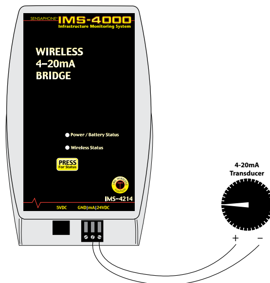
4-20mA Transducer using 24VDC power supply
