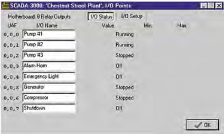
Figure 7: I/O Points Status screen (outputs)
