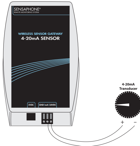
4-20mA Transducer using 24VDC power supply
