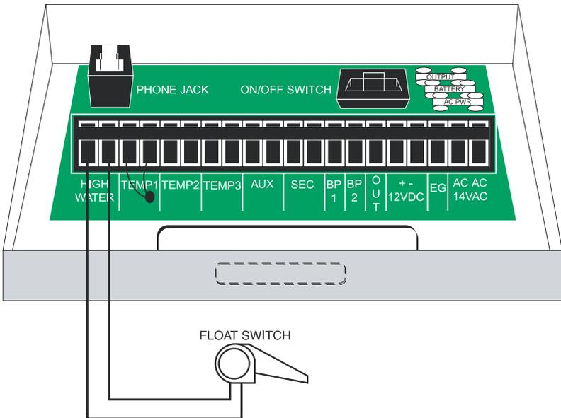
*Fig. 2.3 Connecting the High Water Float Switch*
