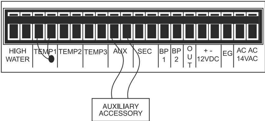
Fig. 2.7 Connection to the Auxiliary Input
