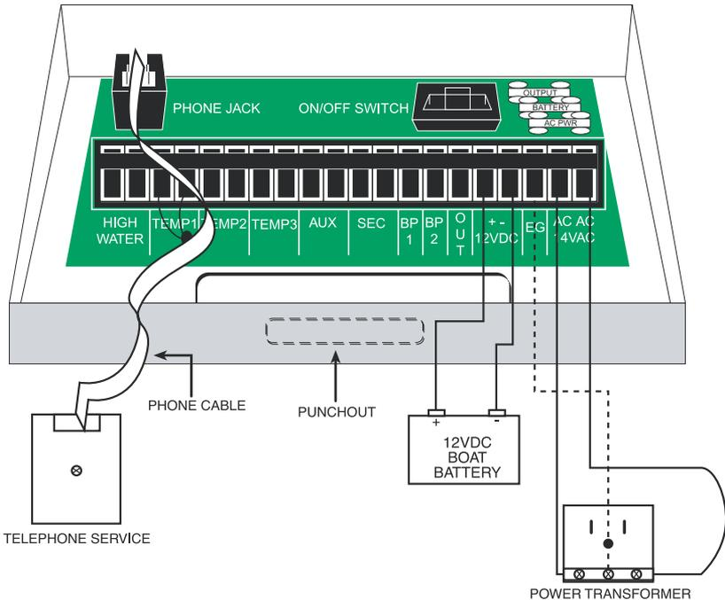
Fig. 2.2 Connecting Power and Telephone Service
