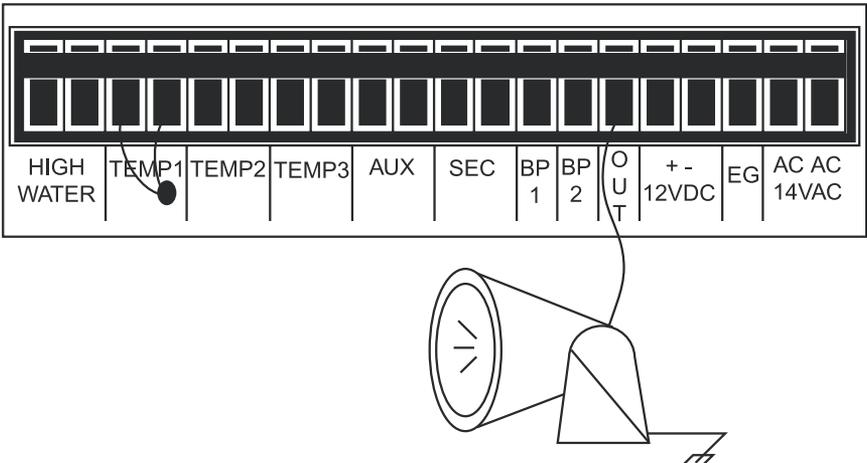
Fig. 2.8 Connecting a Strobe Light to the Output
