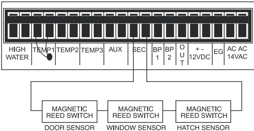
Fig. 2.6 Connecting Accessories to the Security Input
