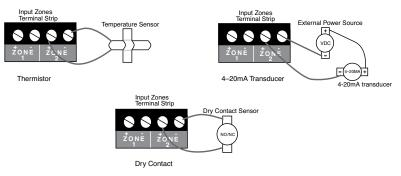
Figure 5: Different Sensor Types connected to the Terminal Block
