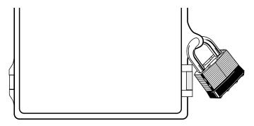
Figure 2: Locking the Enclosure
