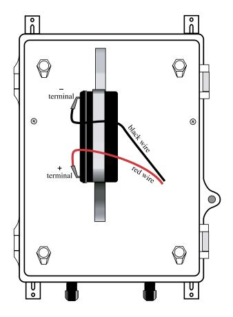
Figure 1: Back-up Battery placement
