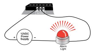
Figure 1: Relay output connected to alarm
