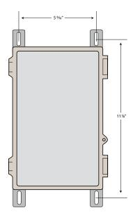
Figure 1: Mounting Dimensions
