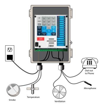
Figure 4: Typical connections from 1800
