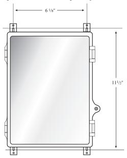
Figure 1: Mounting Dimensions
