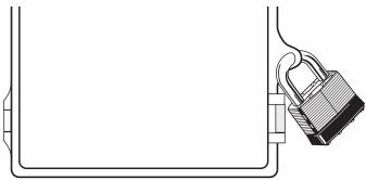
Figure 2: Locking the Enclosure
