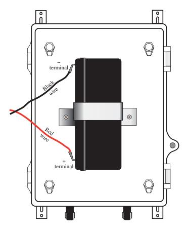
Figure 1: Back-up Battery placement
