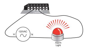
Figure 1: Relay output connected to alarm
