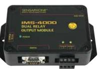
The IMS-4310 Dual Relay Output Module allows you to control two devices from any IMS-4000 Host or Node. Each output may be controlled either manually or automatically. Each output has the option of providing either a dry relay contact or 12VDC power. Two switches located inside the device select the output type.
