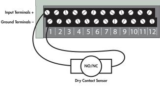
Wiring a Dry Contact Sensor
