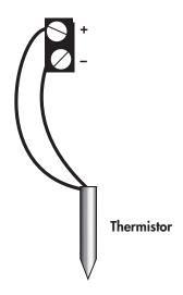
Wiring a Temperature Sensor
