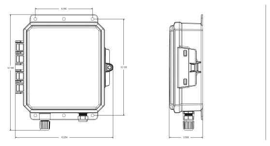
Figure 3: Enclosure mounting dimensions
