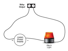
The relay can be controlled manually (via the website or App) or automatically based on specific inputs or alarms. See chapter 3 for details.
