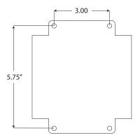
Figure 2: Sentinel mounting dimensions
