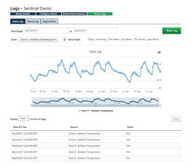
Note that for Normally Open and Normally Closed zone types, the Sentinel will record a "0" when the input is presented with an open circuit and a "1" when the input has a closed circuit. Depending on your sensor and programming, this may represent either a normal or alarm condition.
