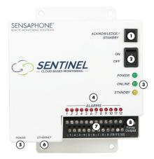
Figure 1: Front Panel Layout of the Sentinel
