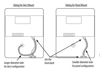
4. Mount the transducer (see the screw hole diagram). Position the transducer vertically.
